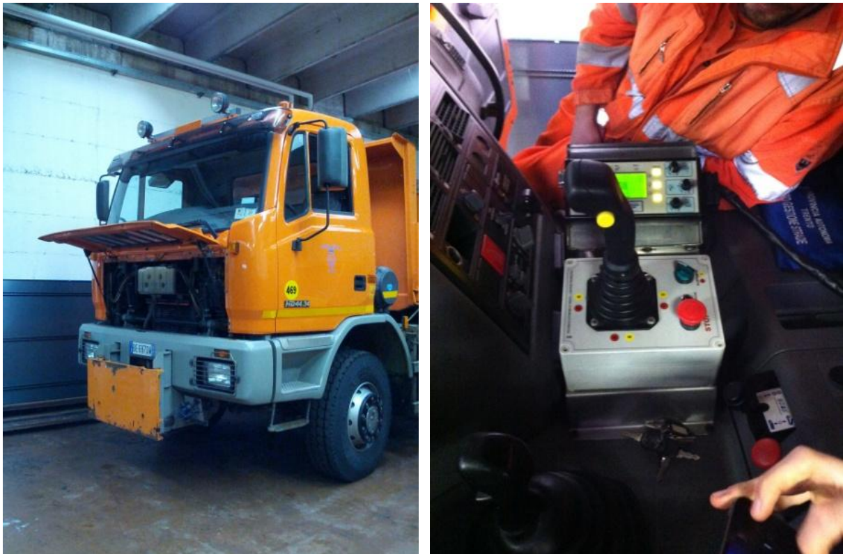
Figure 15: A salt truck and the on-board regulation mechanism for the salt spreading operations.
