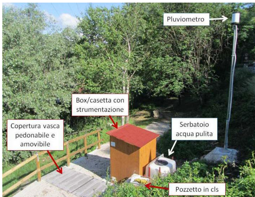
Figure 24: The run-off waters collection and monitoring system installed by the University of Trento in correspondence of the lake of Caldonazzo [5].
