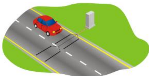
Figure 52: Principle of a piezoelectric traffic detector (source: metrocount.com)
