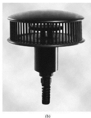
Figure 44: Layout of an electronic anemometer based on ZDT approach [59].
