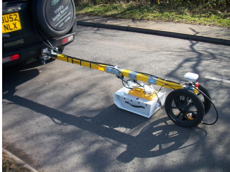
Figure 59: Road construction discontinuities detection through GPR [65].
