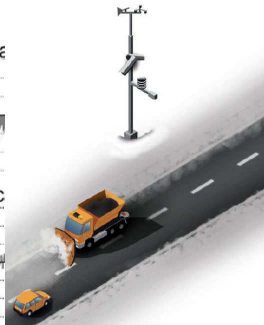
Figure 27: The main elements of a complete road weather monitoring system.
