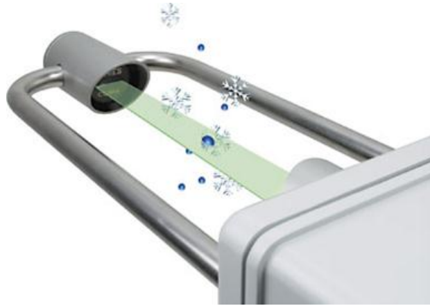
Figure 41: Principle of functioning of an optical disdrometer (source: thiesclima.com)
