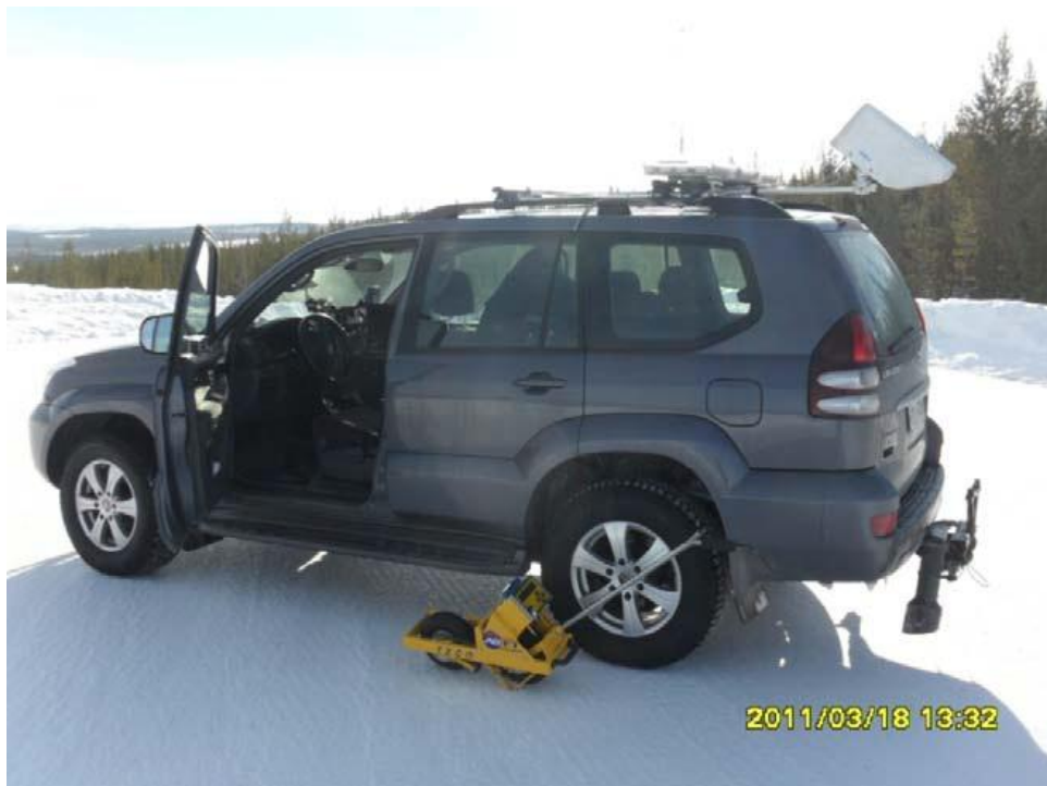
Figure 58: Different friction measurement devices mounted on a probe vehicles [64].
