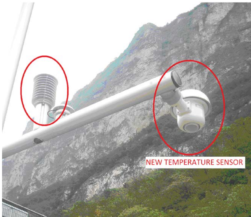
Figure 26: New ventilated temperature sensor (right side) next to the existing air temperature probe.
