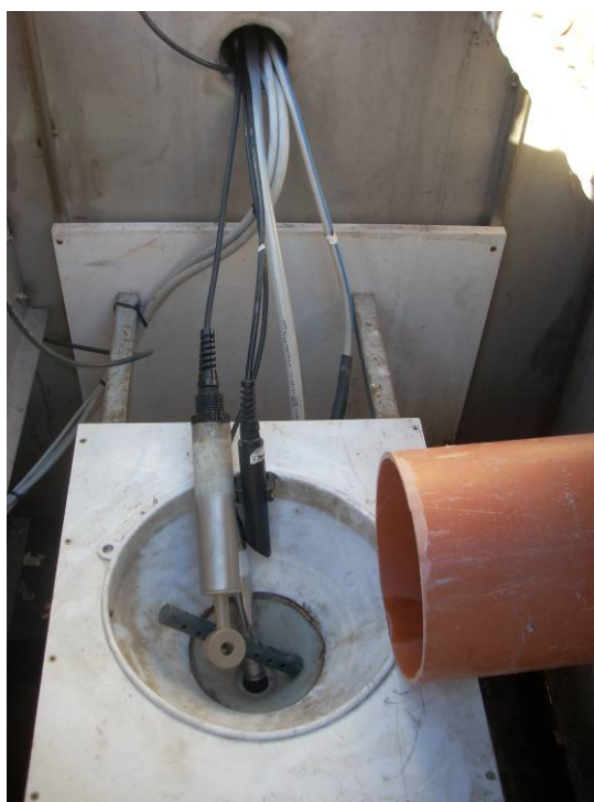
Figure 30: Runoff water collection and monitoring system - sensors for in-situ monitoring of water quality.
