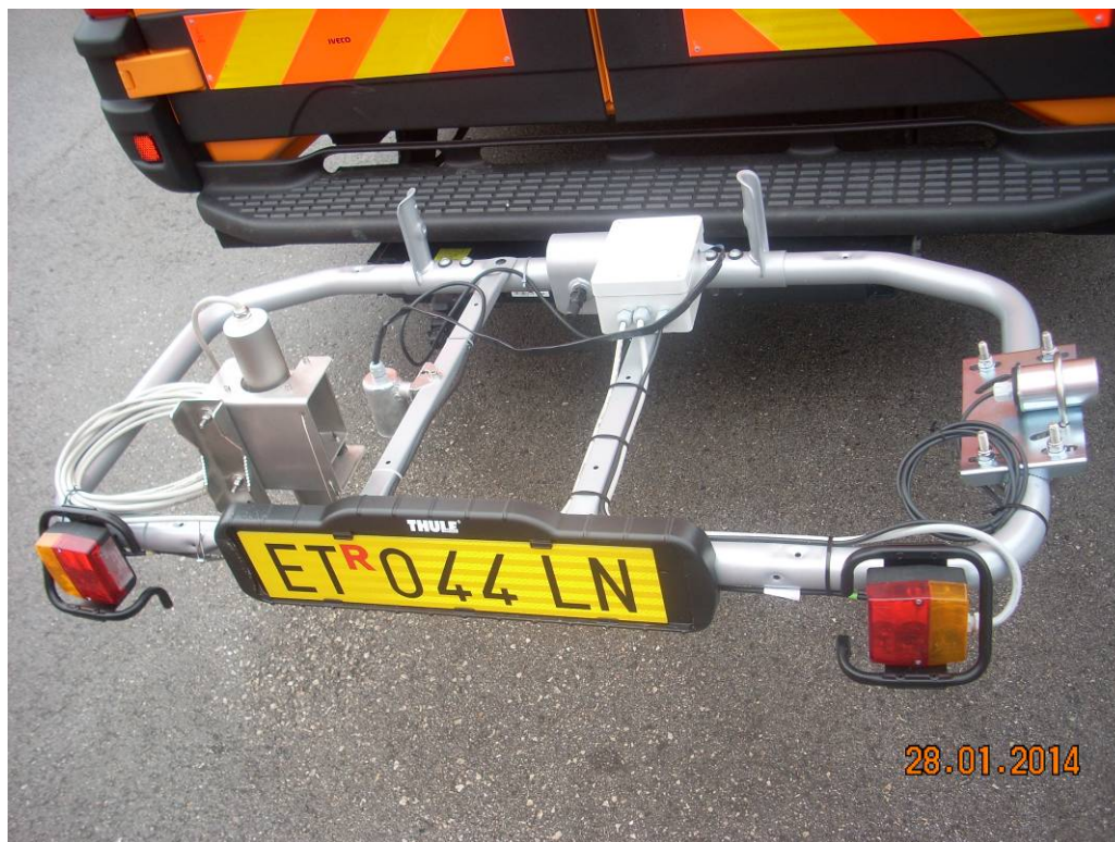
Figure 35: Mobile RWIS station prototype used during first field session activities during winter season 2013/2014.
