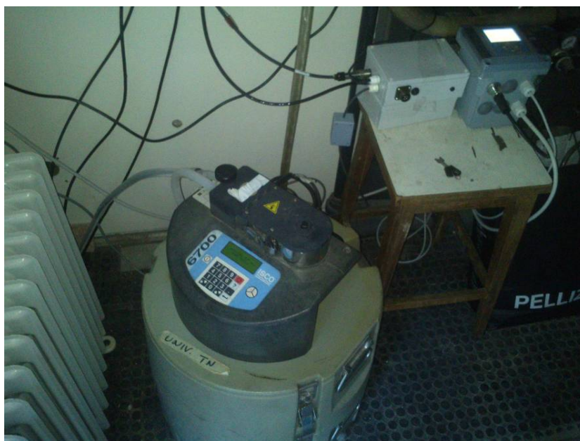
Figure 31: Runoff water collection and monitoring system - automatic sampler and electronic instrumentation to record and transmit data.
