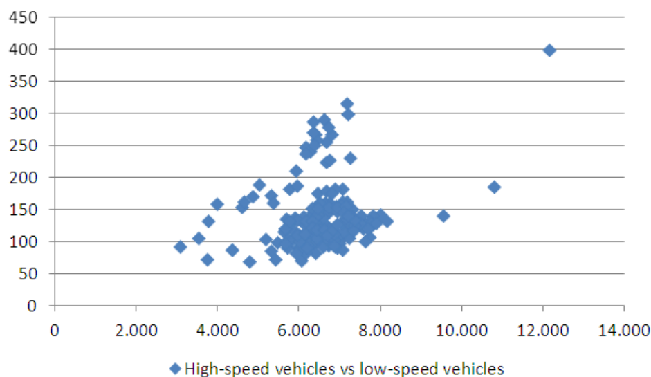
Figure 4: The scatterplot of high-speed and low-speed vehicles in the traffic monitoring point of Salorno (with low speed vehicles classified as those vehicles traveling at speed lower than 60 [km/h]).
