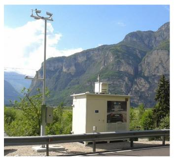
Thanks to the installation of road weather stations and an environmental monitoring site for air and water matrixes. CLEAN-ROADS is able to provide several information such as conditions of the road. air temperature, precipitation events, traffic levels. run-off waters quality and air pollution.
